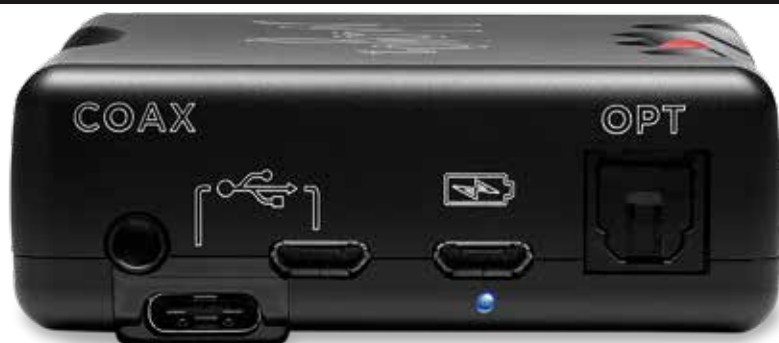
ABOVE: The Micro-USB port is joined by a new USB-C input on the Mojo 2 (up to 768kHz/32-bit and DSD256). Another Micro-USB socket handles battery charging, alongside a 3.5mm S/PDIF coaxial socket with Toslink optical insert. Dual 3.5mm headphone outputs are included on the opposite side of the case
